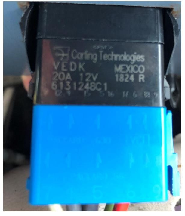
3/28/2020: UHL's crossreferenced a direct replacement switch: International # 6131248C1.Replaced existing failed switch. Removable terminal block was not altered.Mounting plate and switch were returned to operating position on dash.Fan responded properly and reliably through six OFF/LO/HI/LO/OFF cyclings of the switch.
