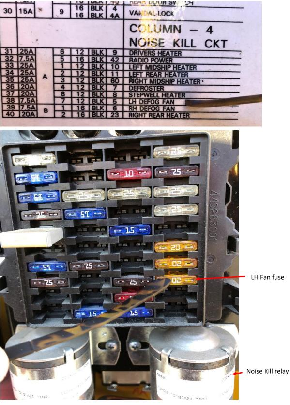
Fuse #38 listed as LH DEFOG FAN, 7.5A. Acutal device is 20A.According to fuse block schedule there should be separate 7.5A fuses for two defog fans.12VDC power consistantly available at fuse #38 with NOISE KILL switch ON.
